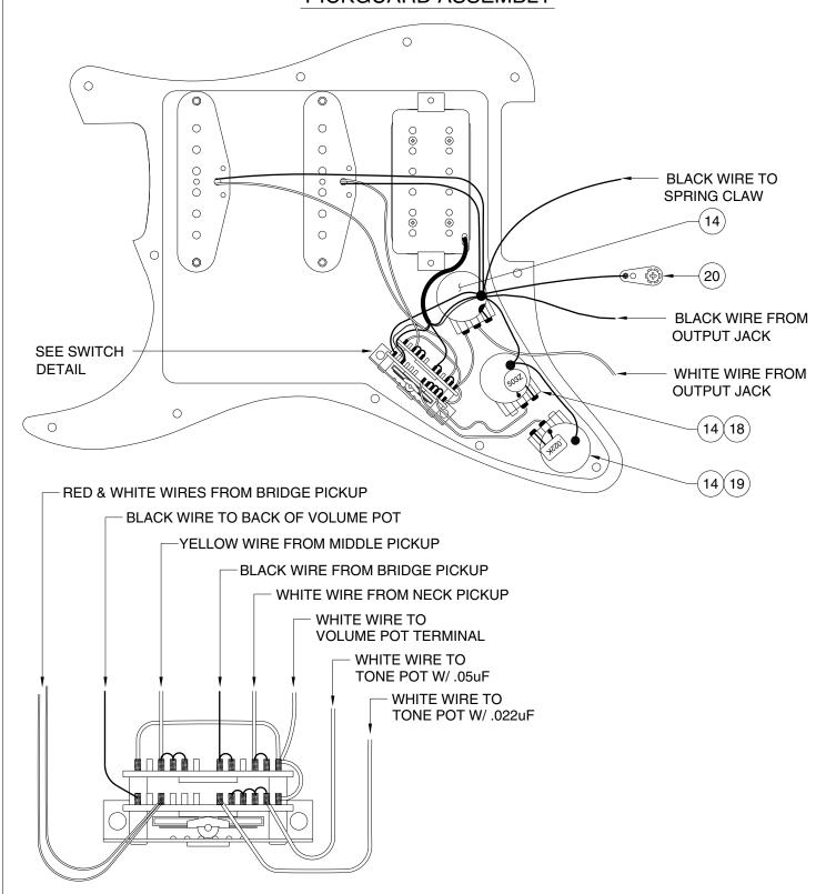
SWITCH WIRING N.T.S.
